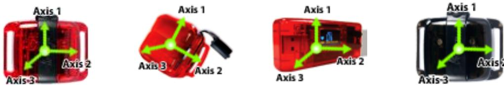
FIGURE 77 - AXIS DEFINITIONS FOR ACTIGRAPH DEVICES
