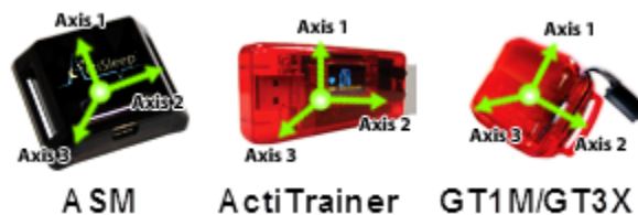
Figure 2 – ASM, ActiTrainer, GT1M, and GT3X axis orientation
