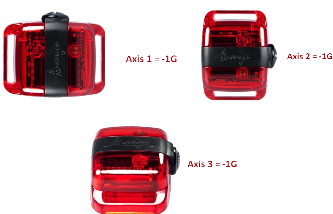
Figure 1 – GT3X+ Axis Orientation
